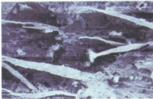
Electron micrograph of Rosette Gault's paperclay body before firing. Courtesy of David Kingery, University of Arizona
